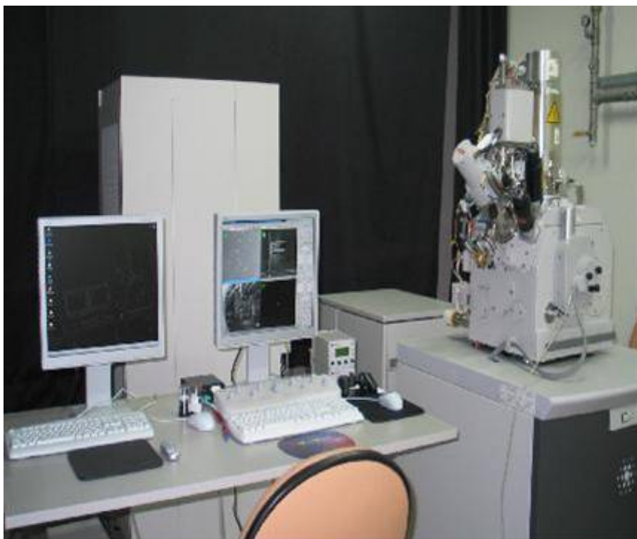
Fig. 3.8 Focused ion beam (FEI Nova 220 FIB).
