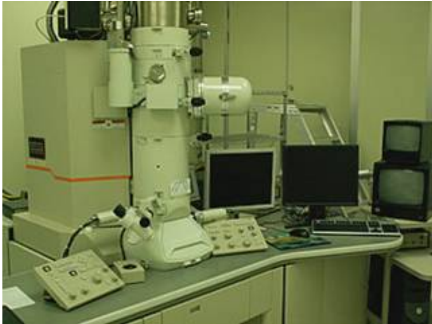
Fig. 3.7 The transmission electron microscopy (Jeol JEM-2100F TEM).
